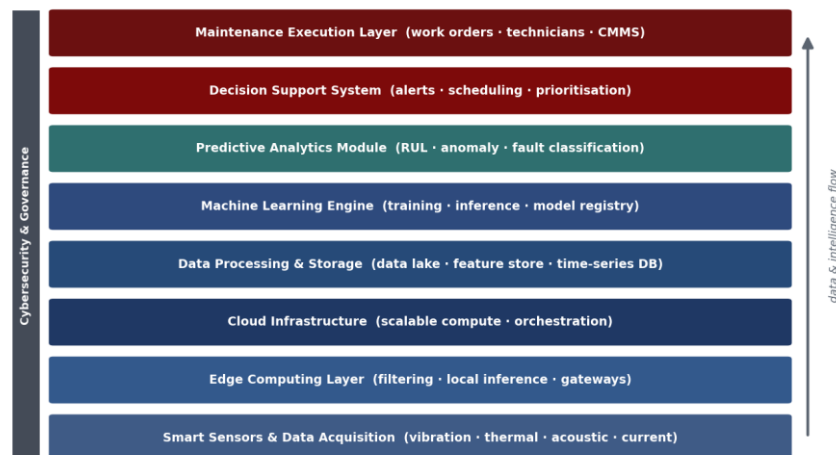
Figure 2: Layered Architecture of the AI-Enabled Predictive Maintenance System
